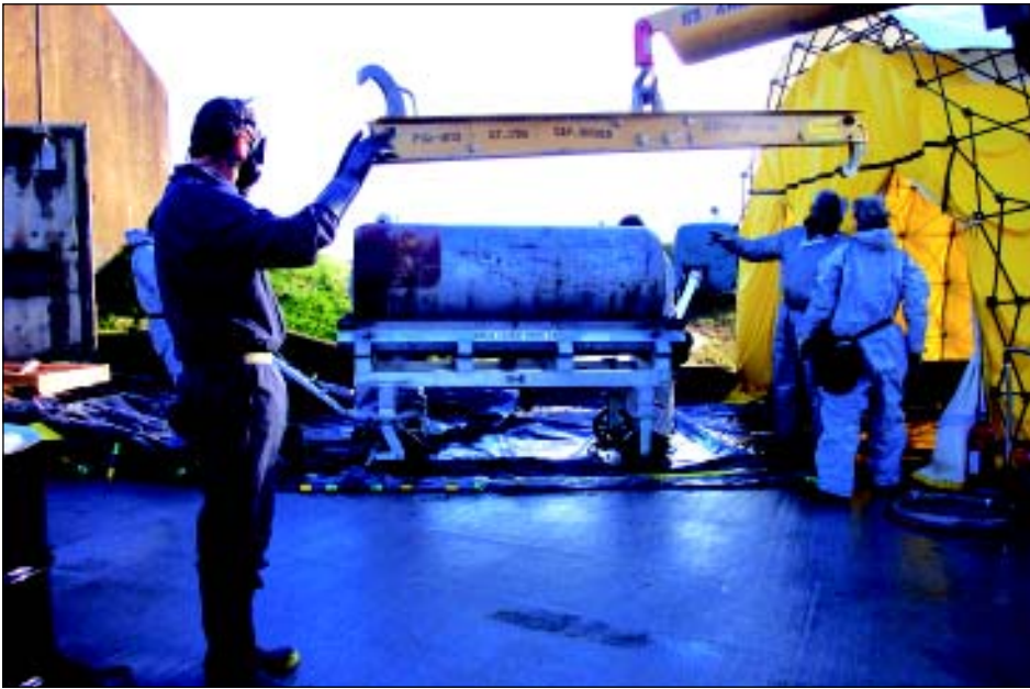
Members of the Technical Escort Unit, a specialized Army unit from Pine Bluff, Ark., prepare the BGAD one-ton container (OTC) for the transfer of its contents into two new OTCs. Photo by the Blue Grass Army Depot
